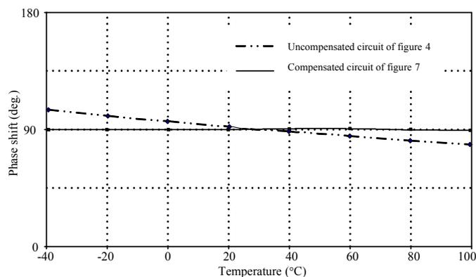
Fig. 10. The variation of the phase shifts  $\phi$  against the temperatures.
