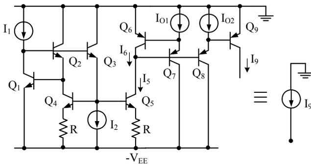
Fig. 6. A tunable temperature dependent constant current source.
