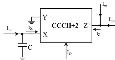
Fig. 4. APF using a single CCCII+2.
