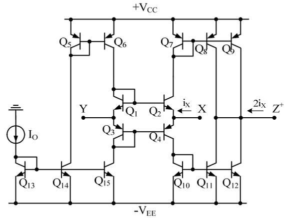
Fig. 3. Schematic implementation of CCCII+2.
