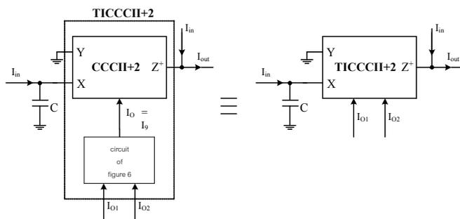
Fig. 7. A temperature-insensitive current-mode APF using a single CCCII+2.
