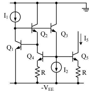
Fig. 5. A temperature dependent constant current source.
