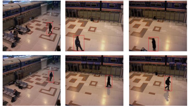
Fig 2. Shows the object tracking using Kalman filter, the object with the red rectangle shows the tracked object.
