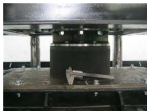
Fig. 4. Photo of the HDRB for RTHS.
