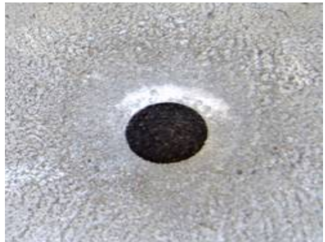
Fig. 4 (b) Machined hole at 15 volts D.C. supply current, (NaCl + HCl : 100g/l + 20ml/l) electrolyte concentration, 50 Hz frequency and 3 l/min electrolyte flow rate.
