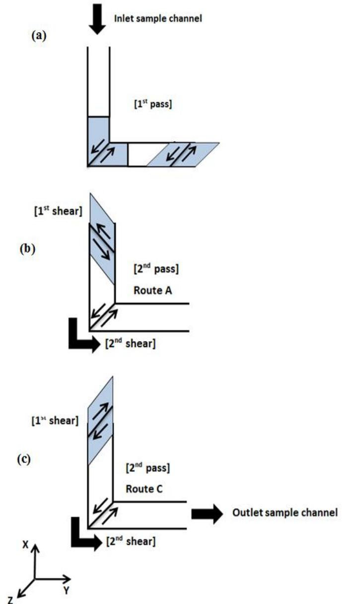
Fig. 3. Interactions of consequent shear deformations in the first and second ECAP pass
