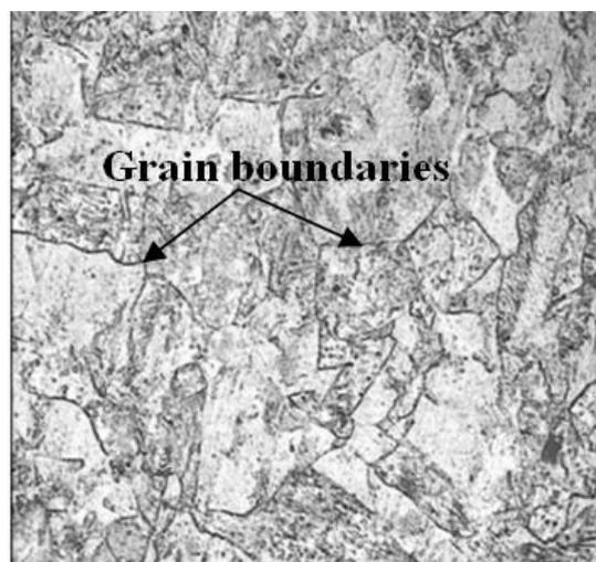
Fig. 2. Optical microscope images of the ECAP copper obtained at 6 passes [17]
