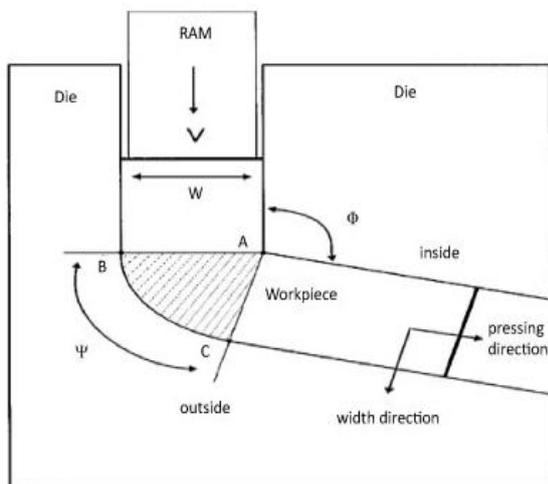
Fig. 1. A schematic view of an equal channel angular pressing angular ECAP [11]
