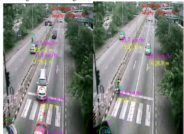
Fig. 4. The Measurement of SSD by ITS
