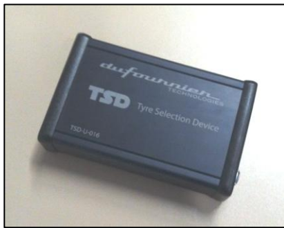
Fig. 2. TSD data acquisition unit.
