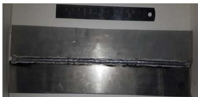
Fig. 2. Specimen fabricated using Pulsed GMAW
