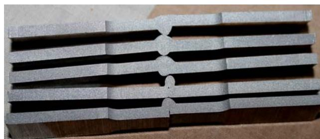
Fig. 3(b). Tensile test samples after Grinding to uniform thickness
