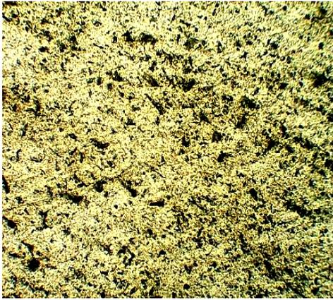
Fig. 4. Micrograph of base metal of a sample fabricated using standard GMAW
