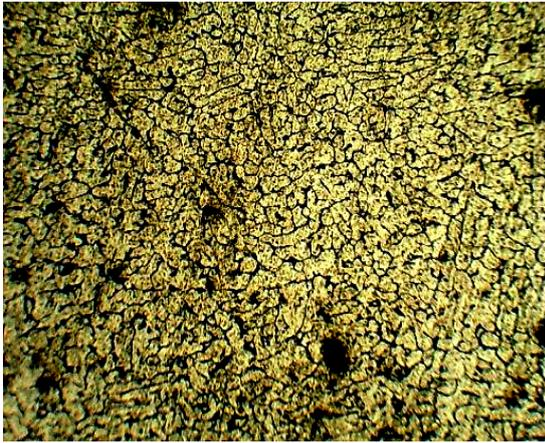
Fig. 8. Micrograph of sample at weld zone fabricated using Pulsed GMAW with arc rotation at 111 A and 19.5 V
