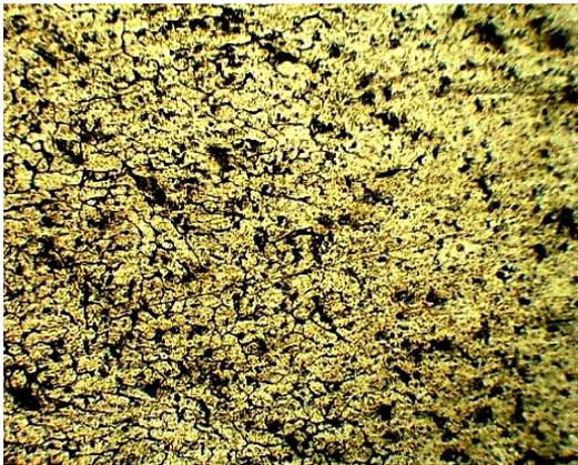
Fig. 5. Micrograph of Heat Affected Zone of a sample fabricated using standard GMAW
