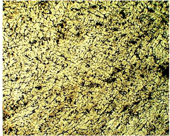
Fig. 6. Micrograph of sample at weld zone fabricated using standard GMAW
