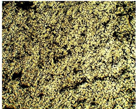
Fig. 7. Micrograph of sample at weld zone using Pulsed GMAW with arc rotation
