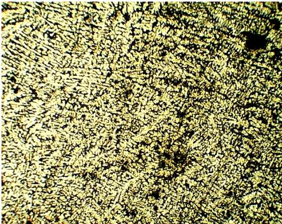
Fig. 9. Micrograph of sample at weld zone fabricated using Pulsed GMAW with arc rotation at 96 A and 12.6 V
