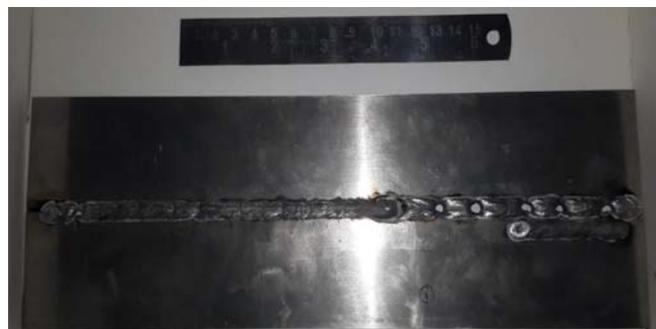
Fig. 1. Specimen fabricated using standard GMAW
