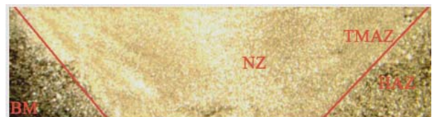
Fig. 5: Macrostructure of the welded joint
