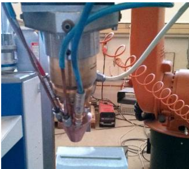
Fig. 1. Experimental setup of the LMD system
