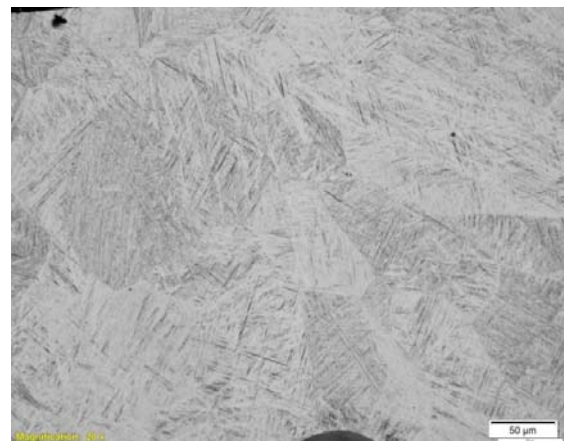
Fig. 4: Microstructure of the deposited zone of sample seven
