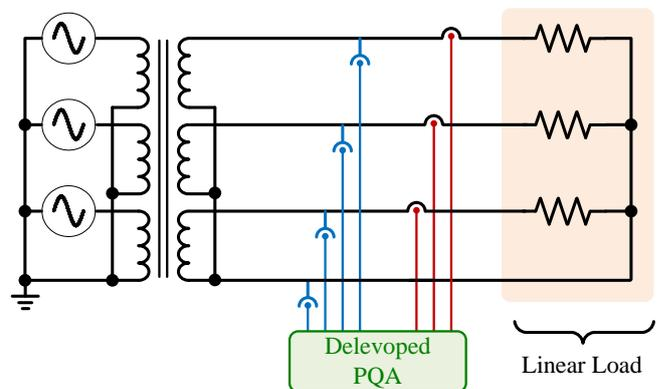
Fig. 6. Electrical diagram of the setup used with a linear load.
