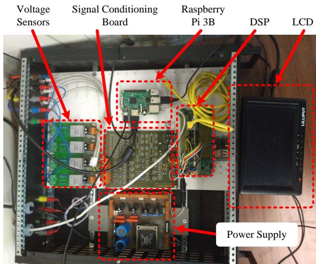
Fig. 4. Developed power quality analyser with integrated electrical energy consumption monitoring system.
