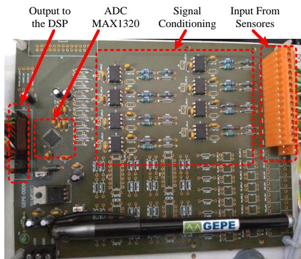
Fig. 3. Developed signal conditioning board with internal ADC.
