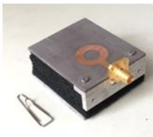
Fig. 2. Fabricated Unidirectional Planar Printed Ring Radiator
