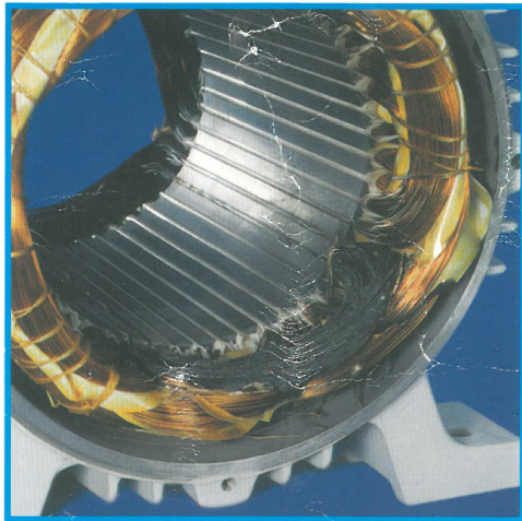
(b) Winding with shorted-coil
