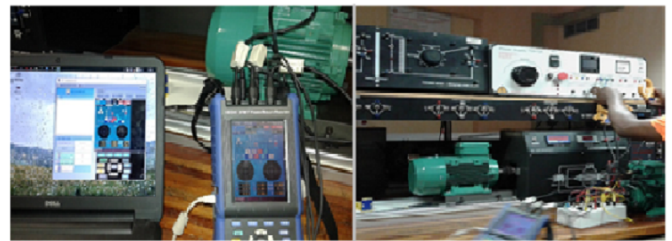
Fig. 2. Experimental Set-up for 1.5kW Induction Motor for data capturing
