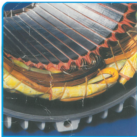
(a) Winding shorted turn-to-turn
