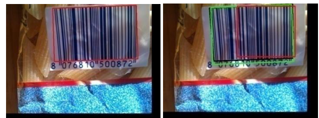
Fig. 12: Sample image for Barcode detection with our method ( J(R,G)=0.960 ) (left image) and result of barcode detection with Creusot (in green) and Zamberletti (in red) (right image)..
