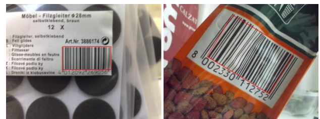
Figure 13: Examples of the detection of blurry and twisted barcodes with J(R,G)=0.933 (left image) and J(R,G)=0.852 (right image).
