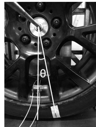
Fig. 5. Definition of the rotation angle \theta .
