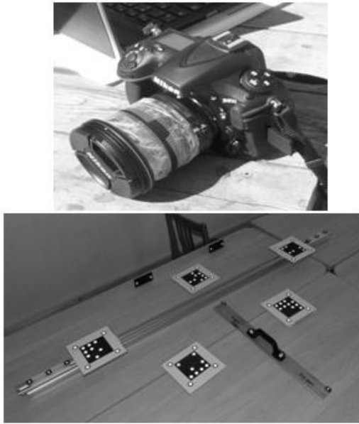
Fig. 5. Digital camera, targets, code marks, scale rule
