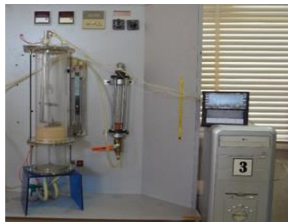
Fig.1 Bubbling fluidized bed apparatus, set up at heat transfer laboratory in IAU, Khomeinishahr Branch
