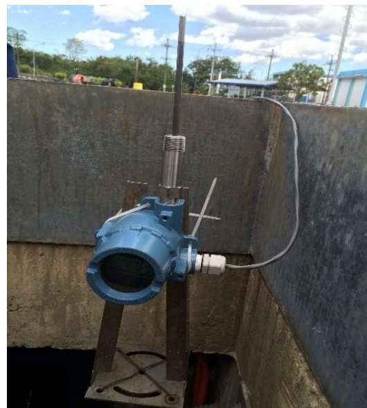
Fig. 3. A thermocouple to measure the temperature on the hot side of the system
