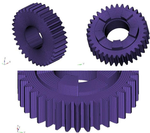
Fig. 3. Mesh Type: Hexahedral, Number of Nodes = 95520, No of Elements = 83080.
