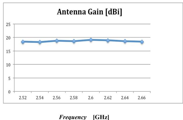
Fig. 5 Antenna gain characteristic
