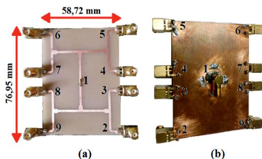
Fig. 8 Antenna feed network ; (a) Front view, (b) Back view
