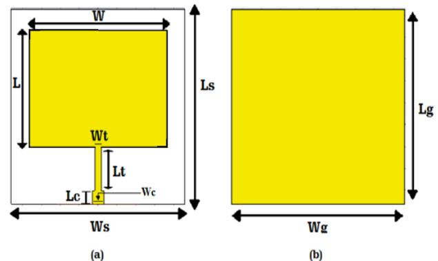
Fig. 1 Rectangular patch microstrip antenna (a) Front view, (b) Back view.
