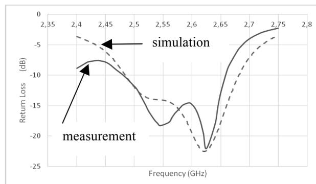
Fig. 10 Antenna Return loss characteristic
