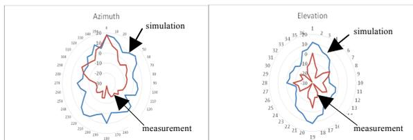
Fig. 12 Antena radiation pattern (Azimuth and Elevation).
