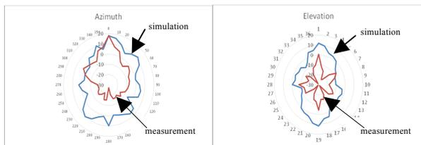
Fig. 12 Antena radiation pattern (Azimuth and Elevation).
