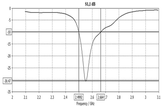
Fig. 4 Antenna frequency characteristics
