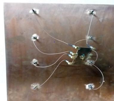
Fig. 9. Uniform feeding network of 8 sub-array antenna
