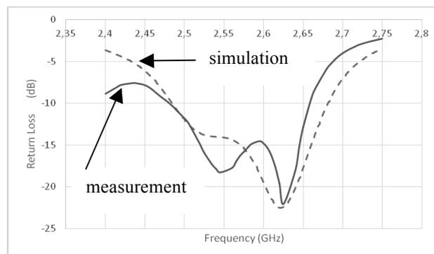
Fig. 10 Antenna Return loss characteristic
