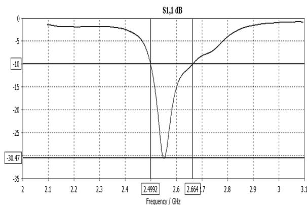
Fig. 4 Antenna frequency characteristics
