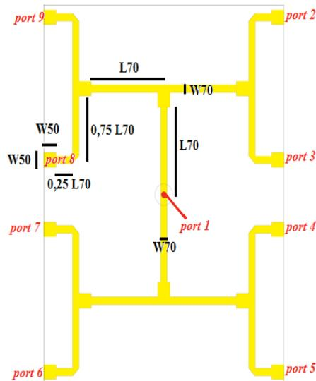
Fig. 3 Power divider for 8-element (4 x 2) sub-array
