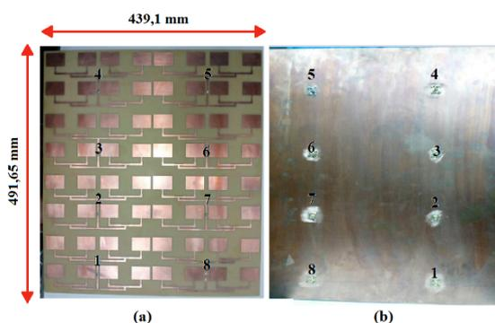
Fig. 7 Fabricated antenna : (a) Front view, (b) Back view
