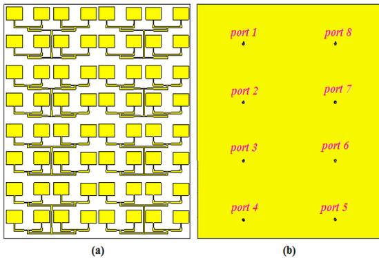
Fig. 2 A 64-element microstrip antenna array with 8 sub-arrays configuration: (a) Front view, (b) Back view.
