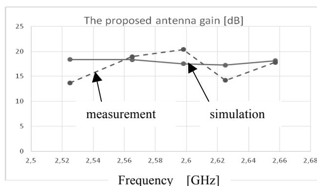
Fig. 11 Antenna gain characteristic
