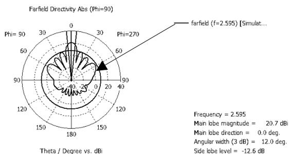
Fig. 6 Antenna radiation pattern (simulation)
