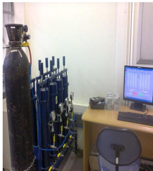
Fig. 1. Oxygen permeability apparatus setup used
