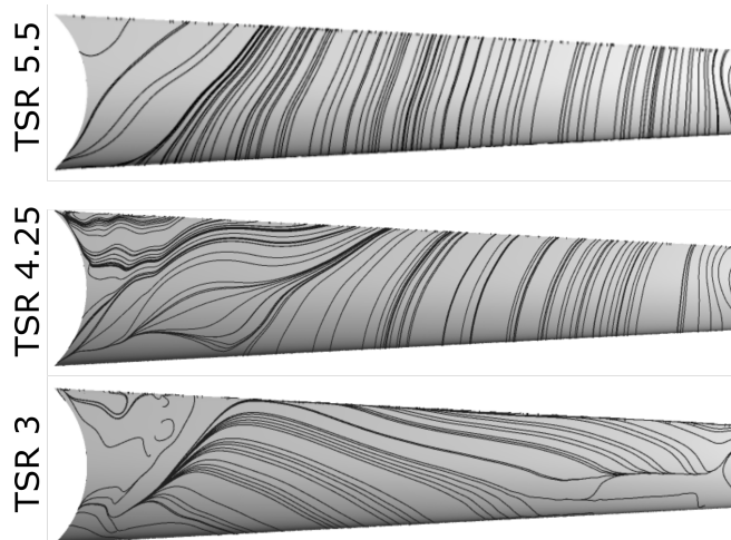
Fig. 13: Blade limit streamline E387(flow direction from bottom to top)
