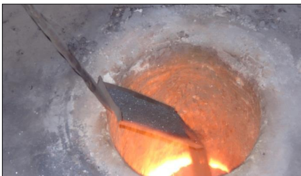
Fig. 3. Feeding SiC micron powder
