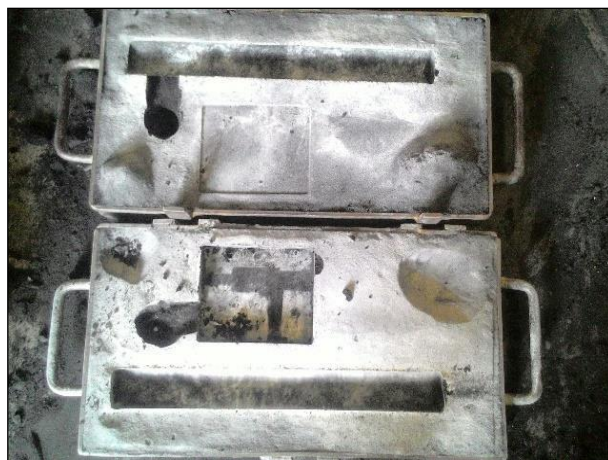
Fig. 5. Sample of sand mold
