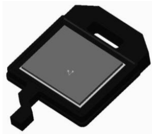
Fig. 2: 3D Model of the SOT package used in the simulation.
