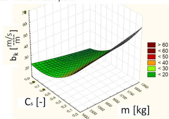
Fig. 6. Relationship between  $b_k$  coefficient,  $C_s$  coefficient and vehicle mass - plane of second order.
