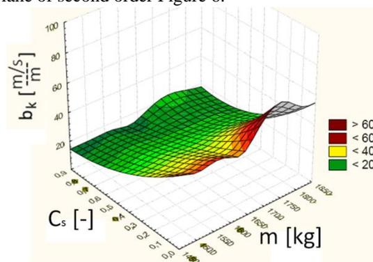
Fig. 5. Relationship between  $b_k$  coefficient,  $C_s$  coefficient and vehicle mass - method of least squares.
