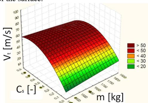
Fig. 4. Relationship between  $V_t$  velocity, coefficient  $C_s$  and vehicle mass  $m$  - plane of second order.
