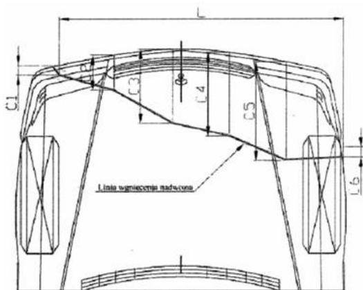
Fig. 9. Measurements of deformation depth.
