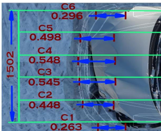
Fig. 10. Measurements of deformation depth.
