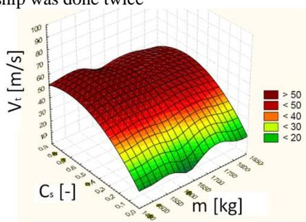
Fig. 3. Relationship between  $V_t$  velocity, coefficient  $C_s$  and vehicle mass  $m$  - method of least squares.
