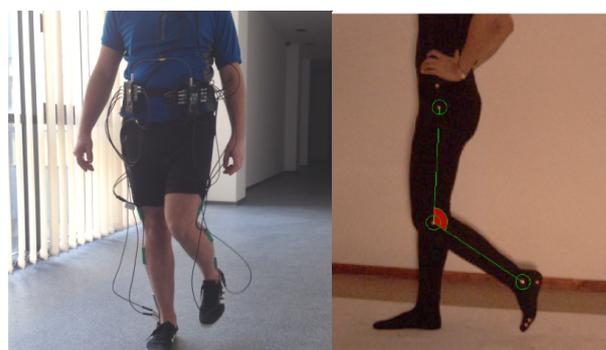
Fig. 7. Subject with wearable sensors and motion processing.
