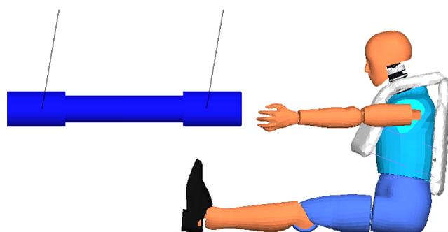
Fig. 6: Thorax impact test virtual model.
