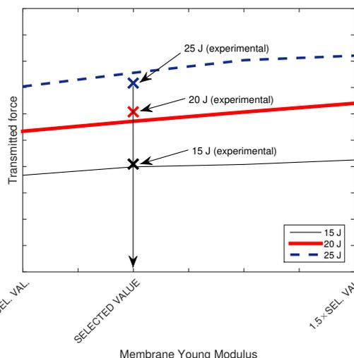
Fig. 5: Effect of membrane Young modulus on the peak of the transmitted force. Cross markers represent the experimental values for each energy level.
