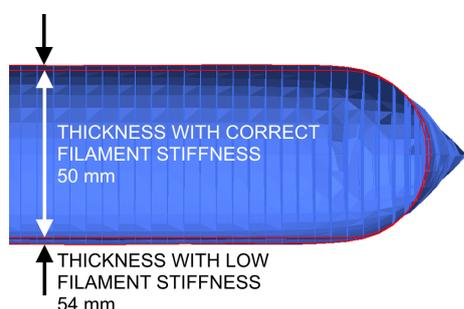
Fig. 4: Difference in inflated airbag geometry caused by different filament stiffness.
