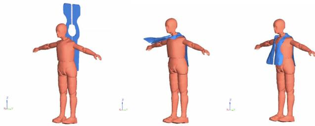
Fig. 7: Fitting process based on accelerations fields to obtain the initial shape of the airbag finite element model – the final step before simulation will involve the addition of the side straps and back connections shown in Fig. 8.
