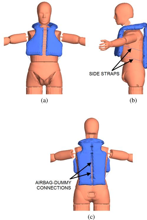
Fig. 8: Airbag finite element model fitted to the Hybrid III 50th dummy: (a) front view; (b) side view (the side straps are highlighted); (c) rear view (the connections between airbag and dummy are highlighted).
