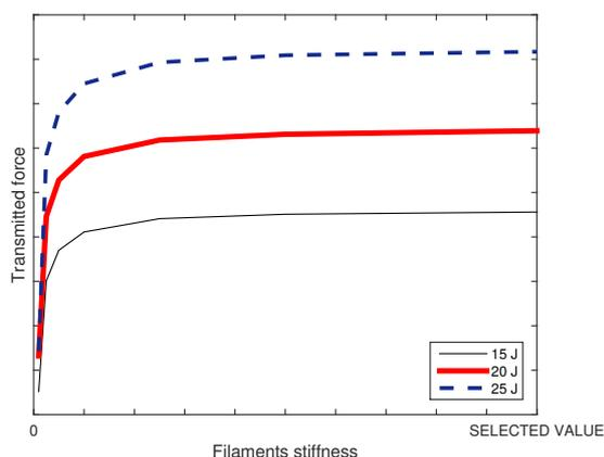
Fig. 3: Effect of filament stiffness on the peak of the transmitted force.
