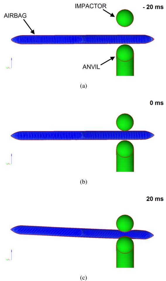
Fig. 2: Drop test simulation: (a) before the impact, (b) at impact and (c) at maximum airbag compression.
