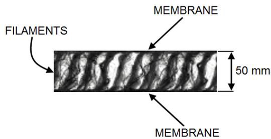
Fig. 1: Airbag membrane and filaments, section view.
