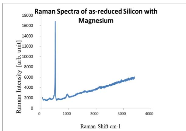
Fig.10 Raman Spectra of Nanostructured silicon from diatomite reduced with Magnesium
