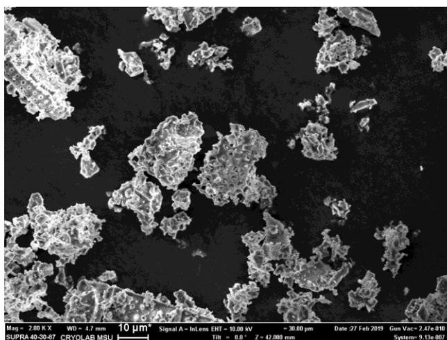
Fig. 5 SEM image of calcined diatomite powder in Air
