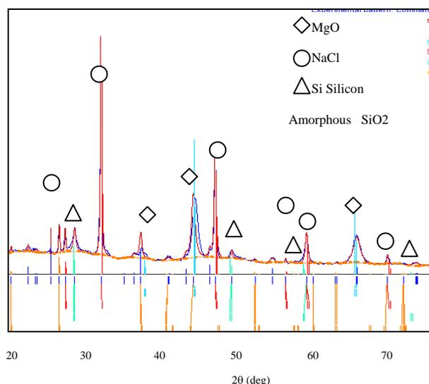
Fig. 8 X-ray diffraction pattern of as-reduced diatomite
