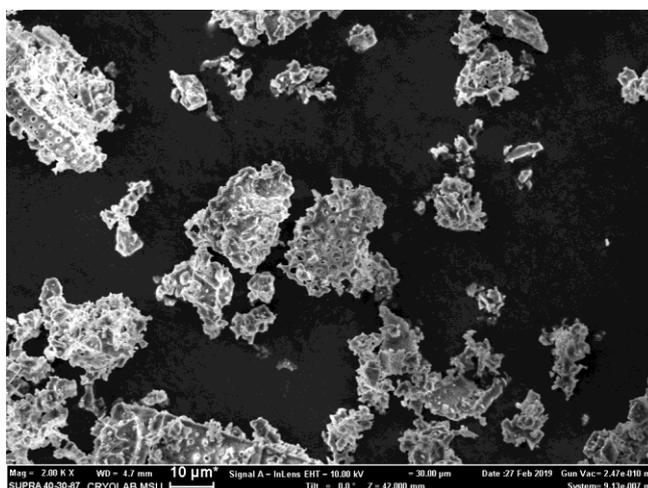
Fig. 5 SEM image of calcined diatomite powder in Air
