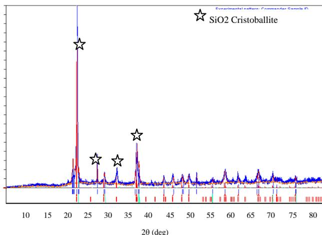
Fig 7 XRD pattern of calcined diatomite powder in Argon
