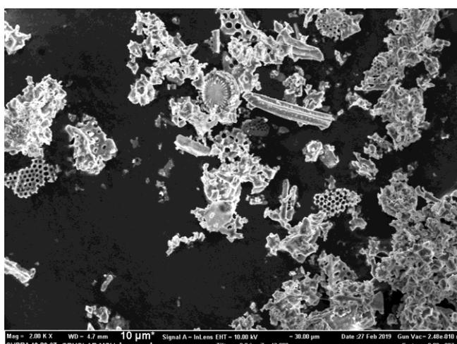
Fig 6 SEM image of calcined diatomite powder under flow of Argon
