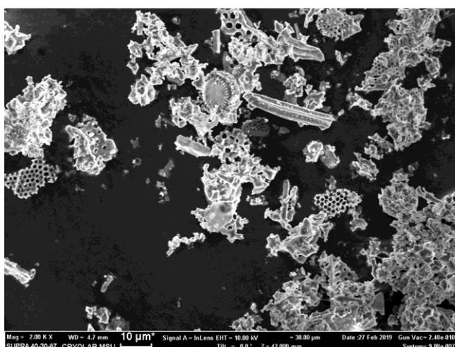
Fig 6 SEM image of calcined diatomite powder under flow of Argon
