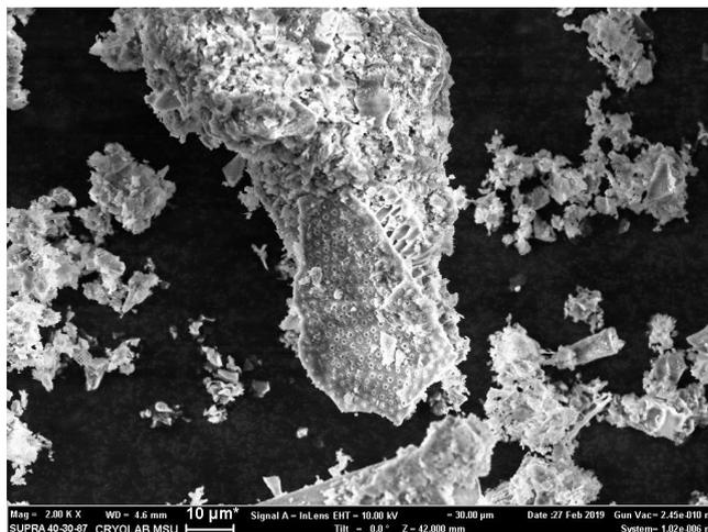
Fig 4 SEM image of diatomite powder from rock sample
