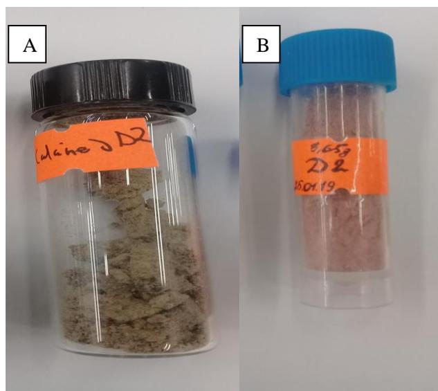
Fig. 3 Colour changes under different calcination condition A) diatomite calcined under flow of Argon B) diatomite calcined in Air
