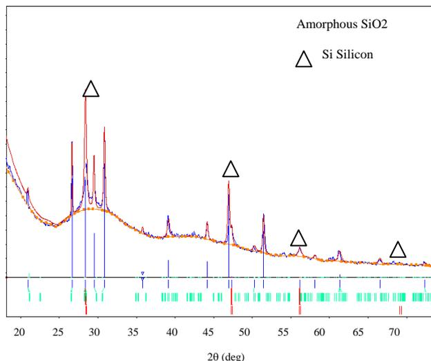
Fig. 9 X-ray diffraction pattern of as-reduced diatomite after etching
