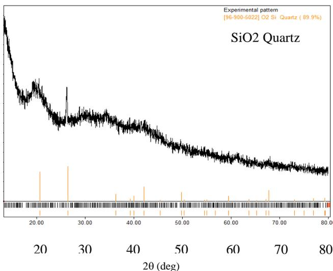
Fig. 1 X-ray diffraction pattern of raw diatomite
