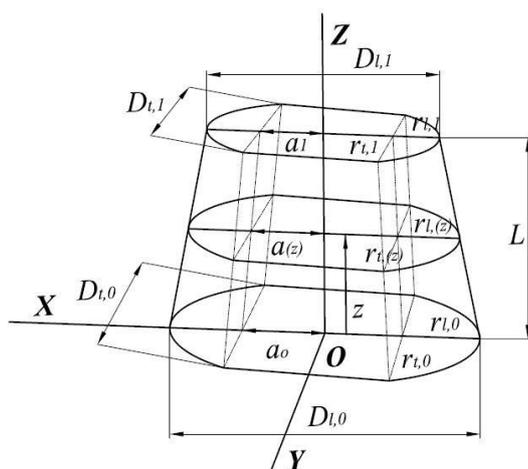
Fig. 3. A right elliptical stadium solid used to model the upper and lower arm.
