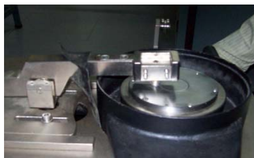
Fig. 1: Wear resistance test on Pin on Disc Tribometer
