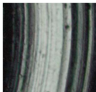
Fig. 2: Wear track of Co-Cr-Mo alloy samples
