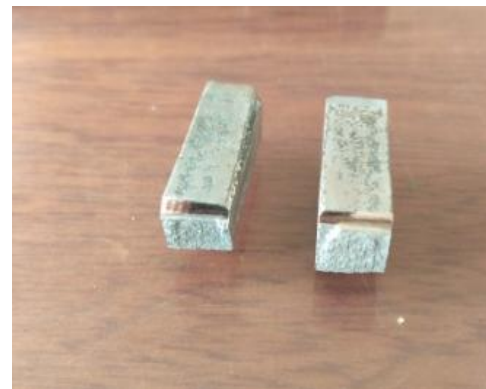
Fig. 2: Fracture of LENS deposited Co-Cr-Mo alloy specimens under impact testing
