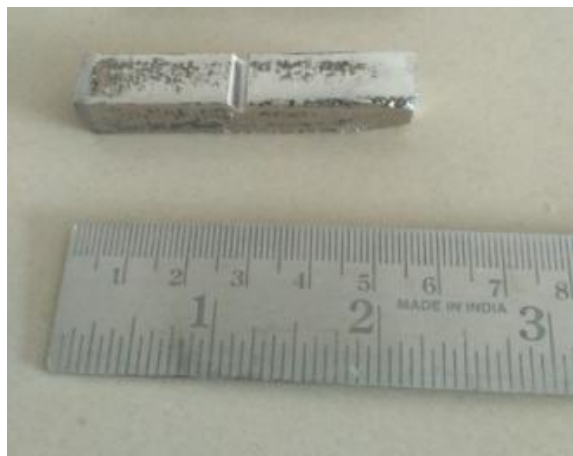
Fig. 1: Impact test specimens fabricated using Laser Engineered Net Shaping as per ASTM Standards
