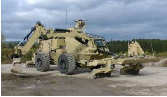
Fig. 1. PEROCC, Pearson eng. route opening and clearing capability (courtesy of Pearson Engineering Ltd ® )
