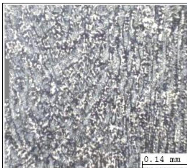
Figure 5 (A) Photomicrograph showing the ferrite morphology in stainless steel weld metal with conventional GMAW process
