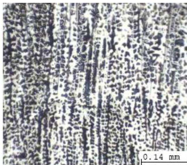
Figure 5 (B) Photomicrograph showing more distinct ferrite morphology in stainless steel weld metal in austenitic matrix of stainless steel weld metal produced with GMAW-EM set up
