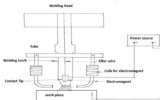
Figure 1 Schematic sketch of GMAW-EM set up
