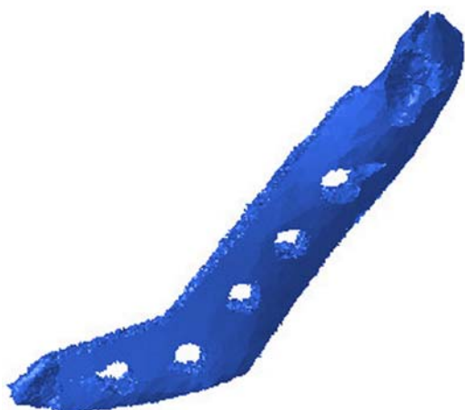
Fig. 3. Topology optimization based TMJ prosthesis
