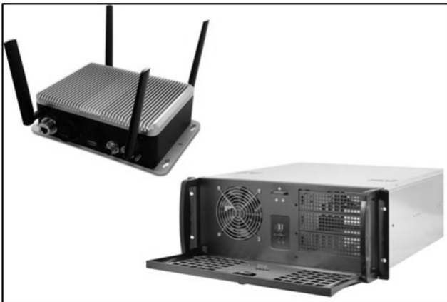
Fig. 7. Communication system (column gateway and RTU)
