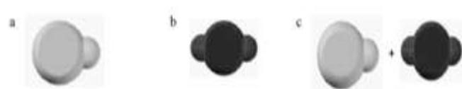
Fig. 3. (a) a two-particle clump used to develop model 1, (b) a 3-particle clump used to develop model 2 and (c) a mixed particle clump used to develop model 3.
