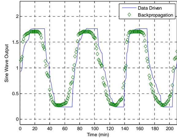
Fig. 8. Data driven vs. feedforward backpropagation for stiction undershoot.
