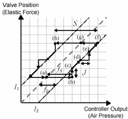
Fig. 2 Typical input-output behavior of a sticky valve adapted from [6].
