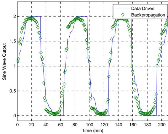
Fig. 10. Data driven vs. feedforward backpropagation for stiction no offset.
