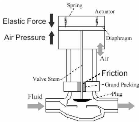
Fig. 1 Structure of pneumatic control valve adapted from [6].
