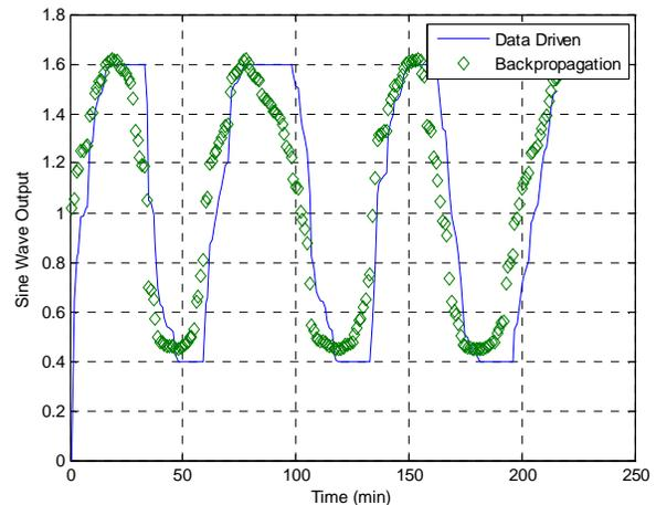
Fig. 6. Data driven vs. feedforward backpropagation for pure deadband case.
