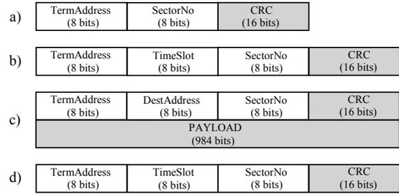
Fig. 2. a) Connection request packet (*con\_req\_packet*), b) Connection response packet (*con\_res\_packet*), c) SDMA/TDMA data packet (*data\_packet*), d) Connection terminate packet (*con\_end\_packet*).
