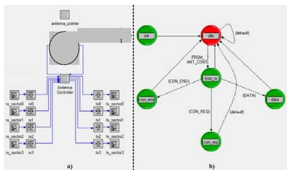
Fig. 4. a) BS node model, b) BS MAC module process model.
