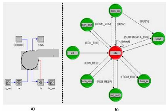
Fig. 3. a) The WT node model, b) The WT MAC module process model.
