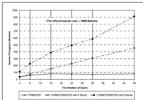
Fig. 9. System throughput for the proposed and regular TDMA/FDD MAC models.
