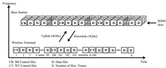
Fig. 1. SDMA/TDMA/FDD frame structure of the proposed MAC protocol.
