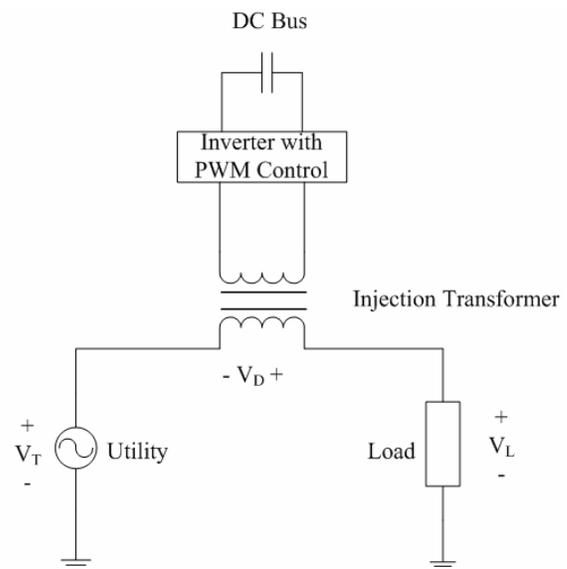
Fig. 1. Conceptual Diagram of one phase of a DVR
