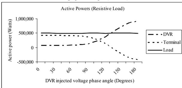
Fig. 9. Active Power variation with injected voltage phase angle (Case II).
