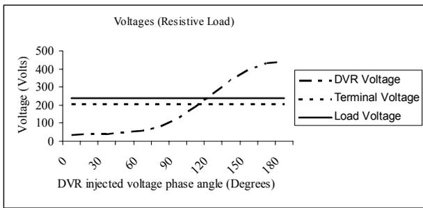
Fig. 7. Voltage variation with injected voltage phase angle (Case II).
