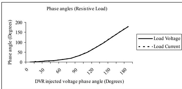
Fig. 8. Phase angle variation of load voltage and current with injected voltage phase angle (Case II).
