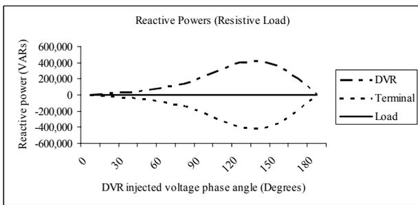
Fig. 10. Reactive Power variation with injected voltage phase angle (Case II).
