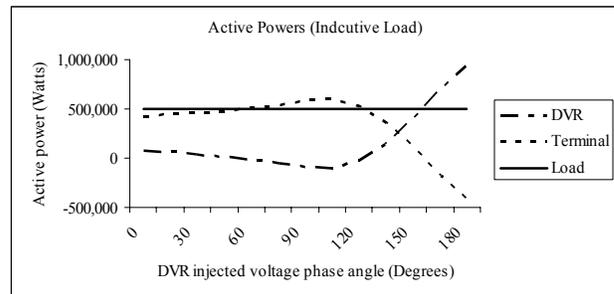
Fig. 5. Active Power variation with injected voltage phase angle (Case I).
