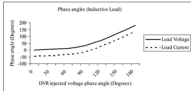
Fig. 4. Phase angle variation of load voltage and current with injected voltage phase angle (Case I).
