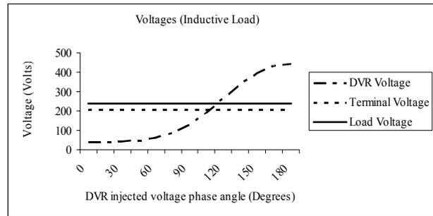
Fig. 3. Voltage variation with injected voltage phase angle (Case I).
