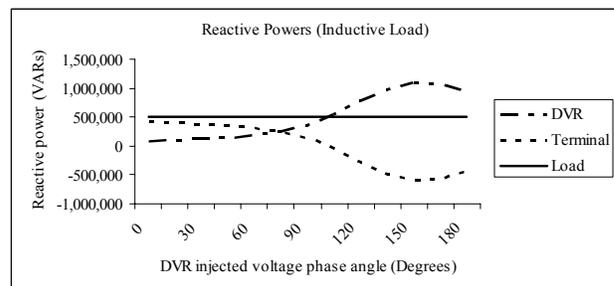
Fig. 6. Reactive Power variation with injected voltage phase angle (Case I).
