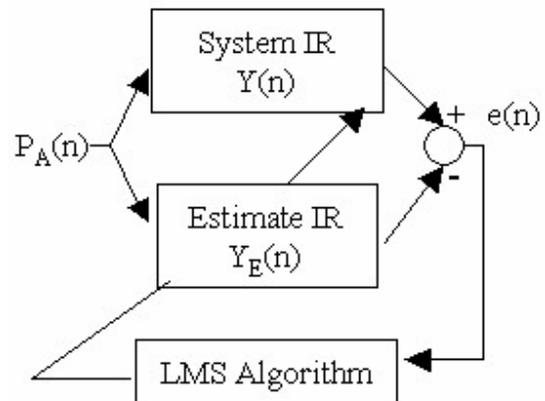
Fig. 2. Identification of Impulse Response of Admittance System Using LMS Algorithm.
