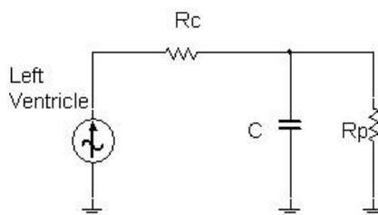
Fig. 1. The 3-element Windkessel model
