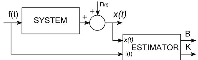
Figure 2: Implementation scheme of the estimator.
