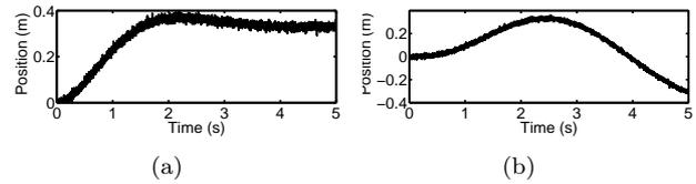
Figure 7: (a) Response of the system to step input and noise in the measure of the mass position. (b) Response of the system to sinusoidal input and error in the measure of the mass position.
