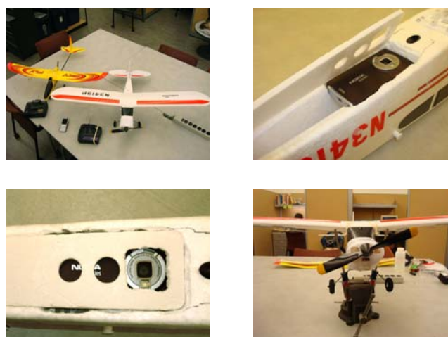
Figure 2: Airplane Modification. Top Left: FlyZone's SkyFly (left) and HobbyZone's SuperCub. Top Right: Phone installed in the housing. Bottom Left: Cover placed on the fuselage. Bottom Right: Balancing of the airplane
