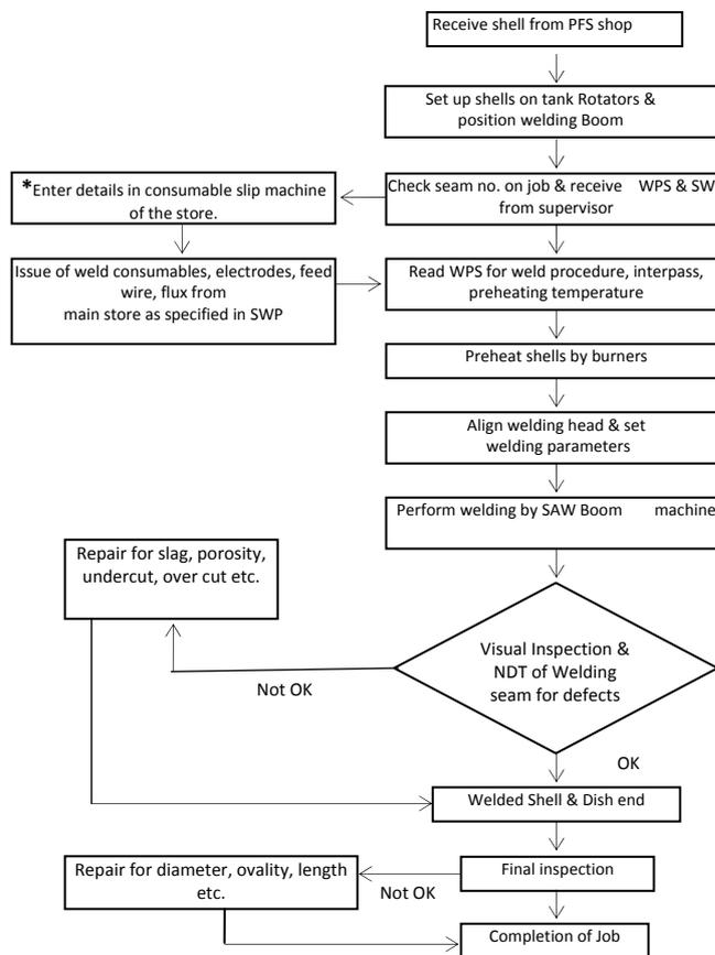
Fig.5 Process Map of SAW Boom machine welding process
