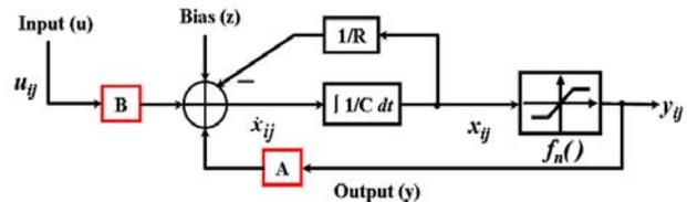
Fig. 1. The block diagram of the Cellular Neural Networks.
