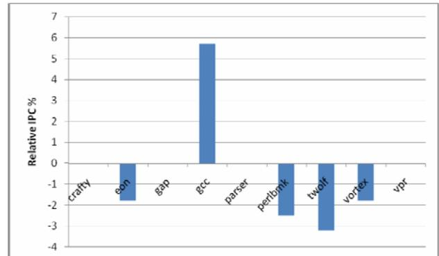
Figure 4: Percentage relative change in IPC when a fault is injected every 1000 conditional branches executed.
