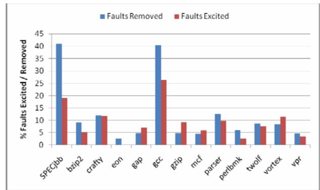
Figure 2: Percentage of faults excited and removed when faults are introduced into BTB
