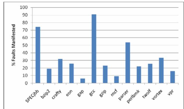
Figure 3: Percentage of faults excited when faults are introduced into branch predictor table
