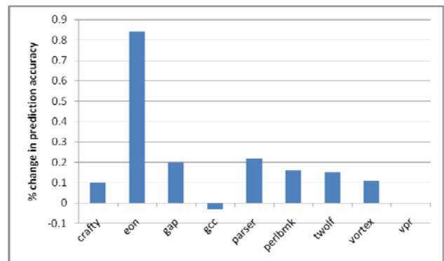
Figure 5: Percentage relative change in branch prediction accuracy when a fault is injected every 1000 conditional branches executed.
