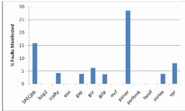
Figure 1: Percentage of faults injected into RAS that are manifested
