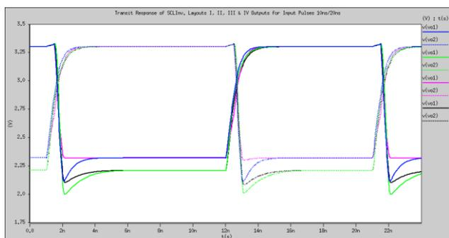
Fig. 9. Outputs of SCL inverter netlist and layouts for 10ns/20ns input pulses.
