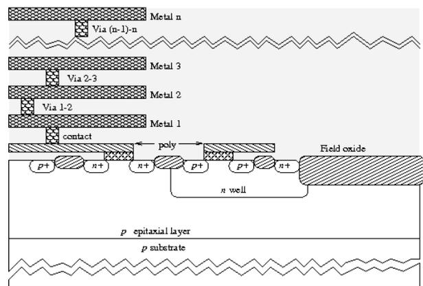
Fig. 3. Interconnection parasitics capacitances among CMOS layers.
