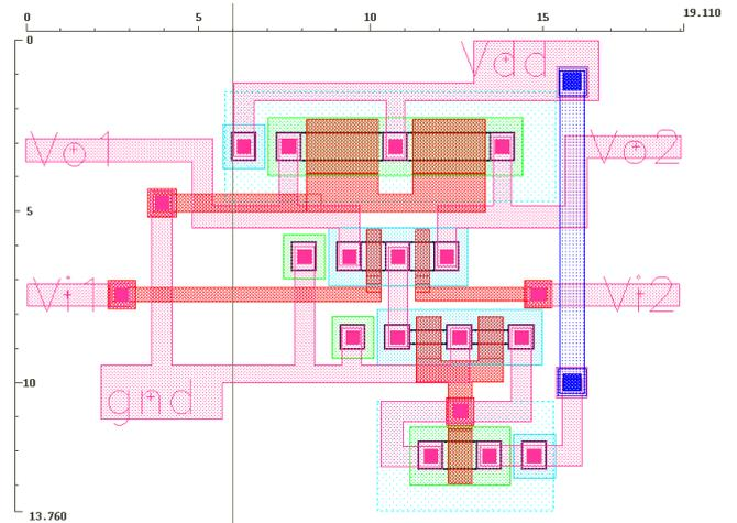
Fig. 6. Comb layout of SCL inverter.
