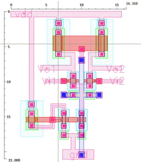
Fig. 4. 1<sup>st</sup> Layout of SCL Inverter.
