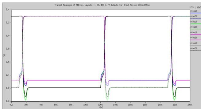
Fig. 8. Outputs of SCL inverter netlist and layouts for 100ns/200ns input pulses.
