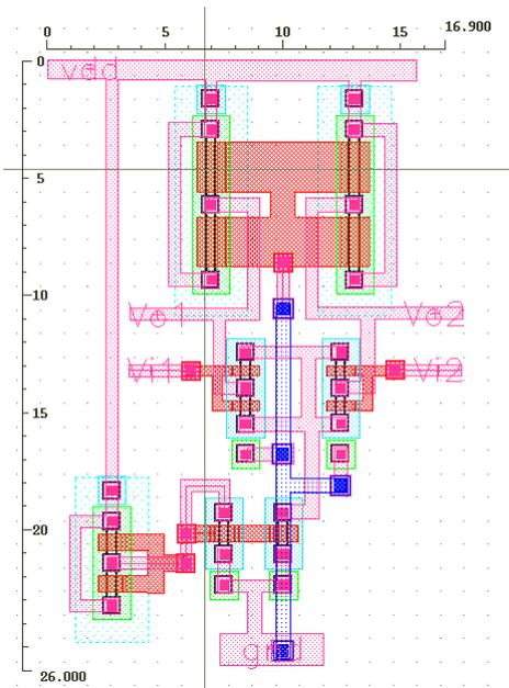
Fig. 5. 2<sup>nd</sup> Layout of the SCL inverter.
