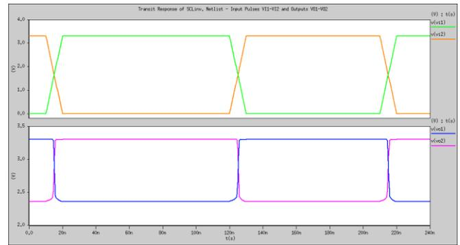
Fig. 2. The Inputs/outputs of SCL inverter netlist
