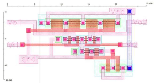
Fig. 7. Fingering and Comb layout of SCL inverter.
