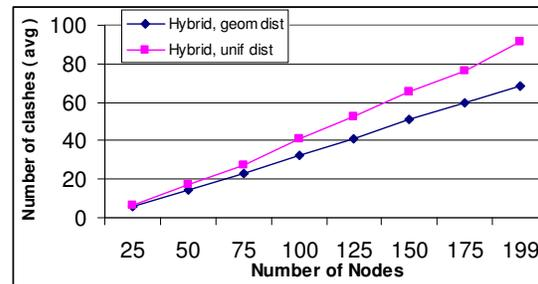
Figure 10. Number of address duplication for hybrid scheme.
