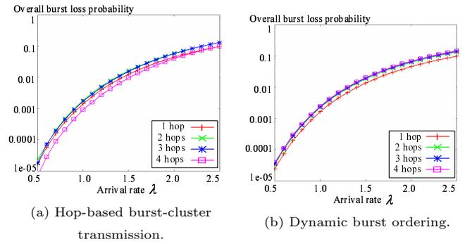
Figure 12: Burst loss probability in the tandem network vs. arrival rate.
