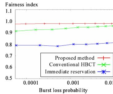
Figure 13: Fairness index in the tandem network vs. overall burst loss probability.
