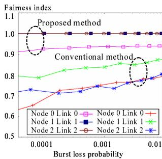
Figure 11: Fairness index vs. overall burst loss probability for each pair of source node and output link.
