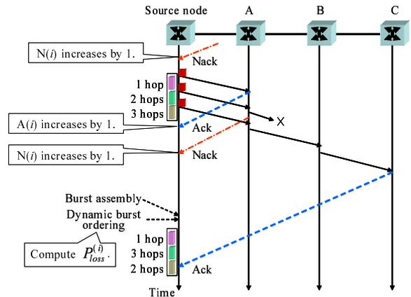
Figure 4: Dynamic burst ordering with ACK and NACK messages.
