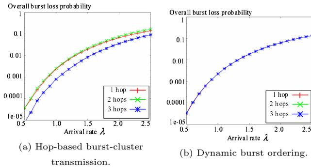
Figure 10: Burst loss probability vs. arrival rate (node 3 and link 2).
