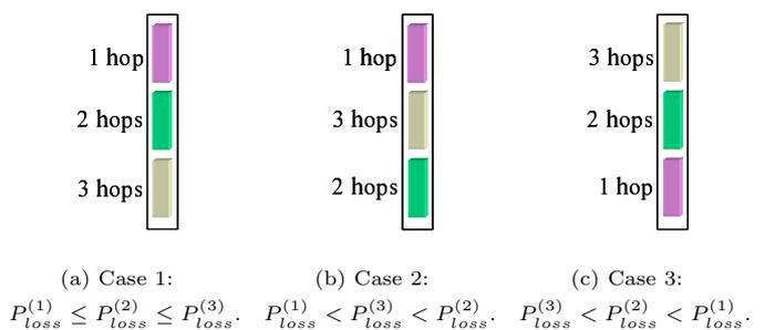
Figure 5: Dynamic burst ordering based on the calculated burst loss probabilities.
