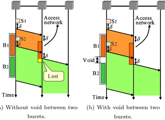
Figure 7: The impact of void on burst preemption.
