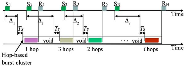
Figure 6: Hop-based burst-cluster transmission with dynamic burst ordering.
