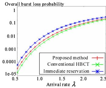
Figure 14: Overall burst loss probability vs. arrival rate.
