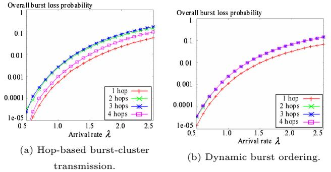
Figure 9: Burst loss probability vs. arrival rate (node 0 and link 0).
