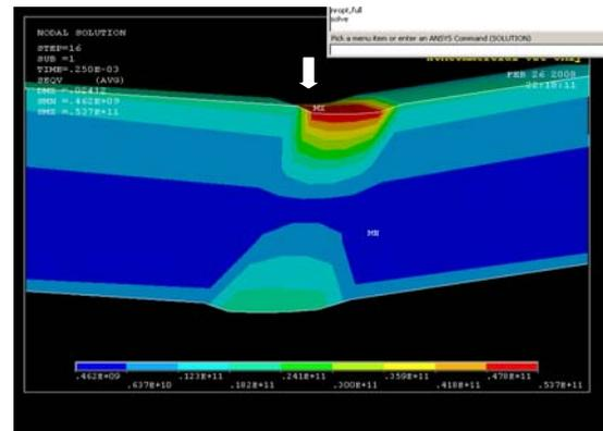
Fig. 9 Stress distribution along the copper wire
