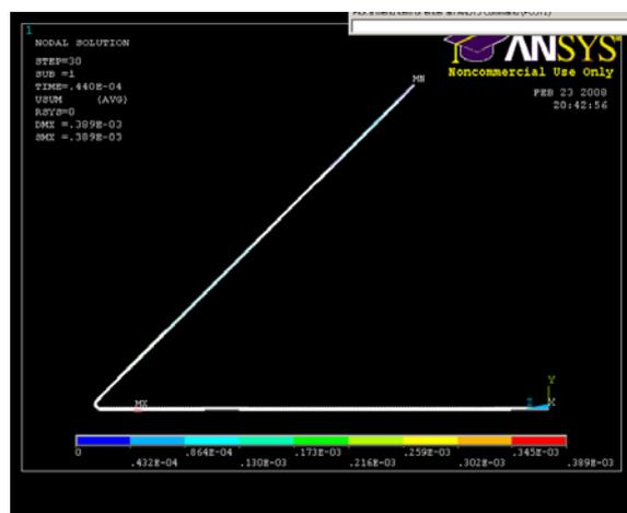
(a) Copper wire deformation at the 44th micro second (the ending time of impulse current)
