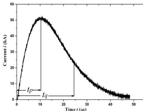
Fig. 2 Input impulse current ( $t_p=10 \mu\text{s}$ ,  $t_q=24 \mu\text{s}$ )
