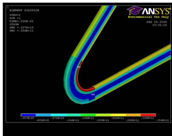
Fig. 7 Current density distribution at the second micro second (Curved angle  $\alpha=45^\circ$  Diameter  $D=1.0mm$ )
