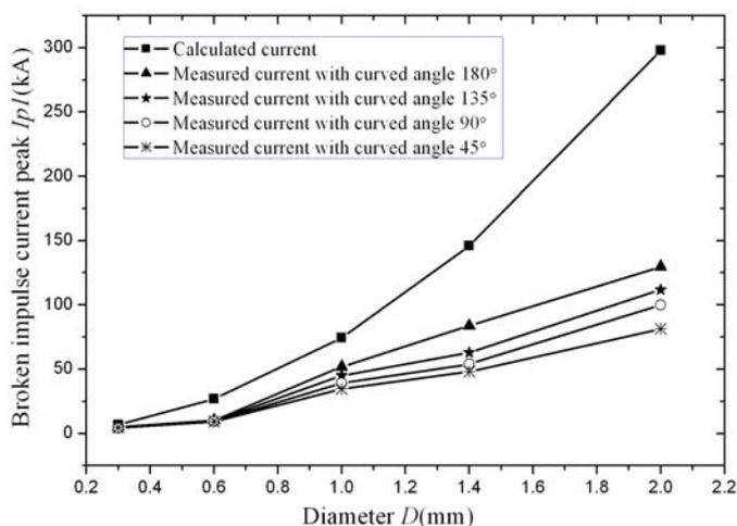
Fig. 4 Breakage characteristics of curved copper wires (impulse peak value versus diameter)
