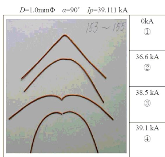
Fig. 3 Breakage process of curved copper wires
