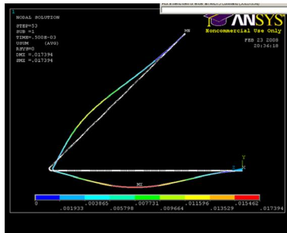
(b) Copper wire deformation at the 500th micro second (this time after the impulse current)
