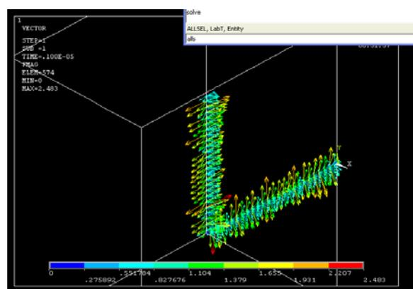
Fig. 6 Magnetic force distribution at the first micro second (Curved angle  $\alpha=90^\circ$  Diameter  $D=1.0mm$ )
